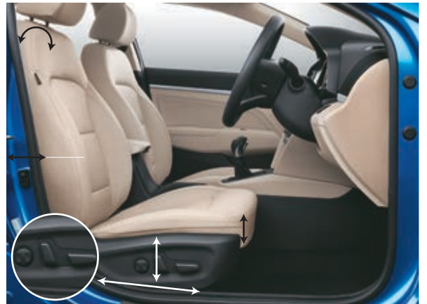
10 Way Adjustable Power Driver Seat with Electric Lumbar Support
