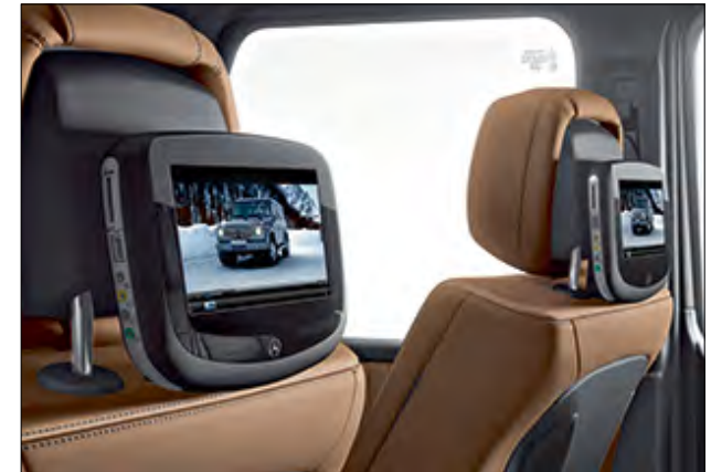
The two displays for the Rear Seat Entertainment System mounted on the front-seat head restraints.
