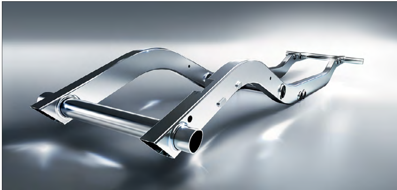
The G-Class is exceptionally stable and durable thanks to its ladder-type frame.
