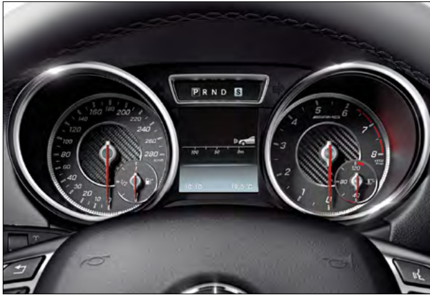
New instrument cluster with carbon fiber background, new pointers and a colour display
