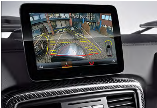
The reversing camera shows the area behind the vehicle during parking.
