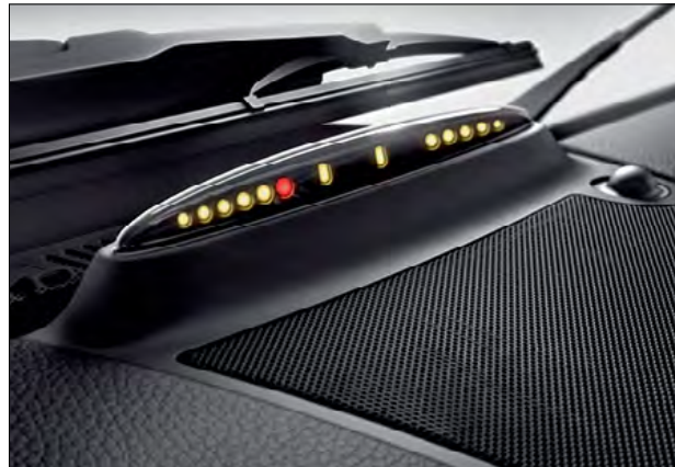
The PARKTRONIC LEDs indicate the distance to the obstacle.
