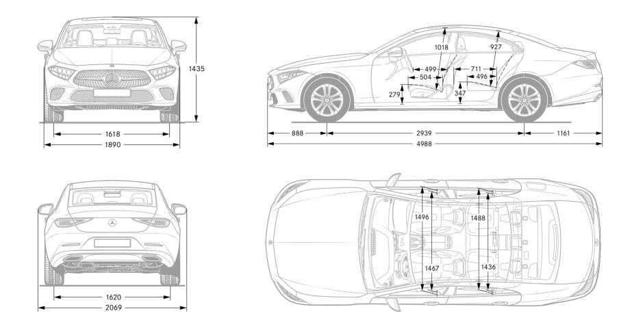
All figures in millimetres. The dimensions shown are median values. They are applicable for unladen vehicles in the standard specification.
