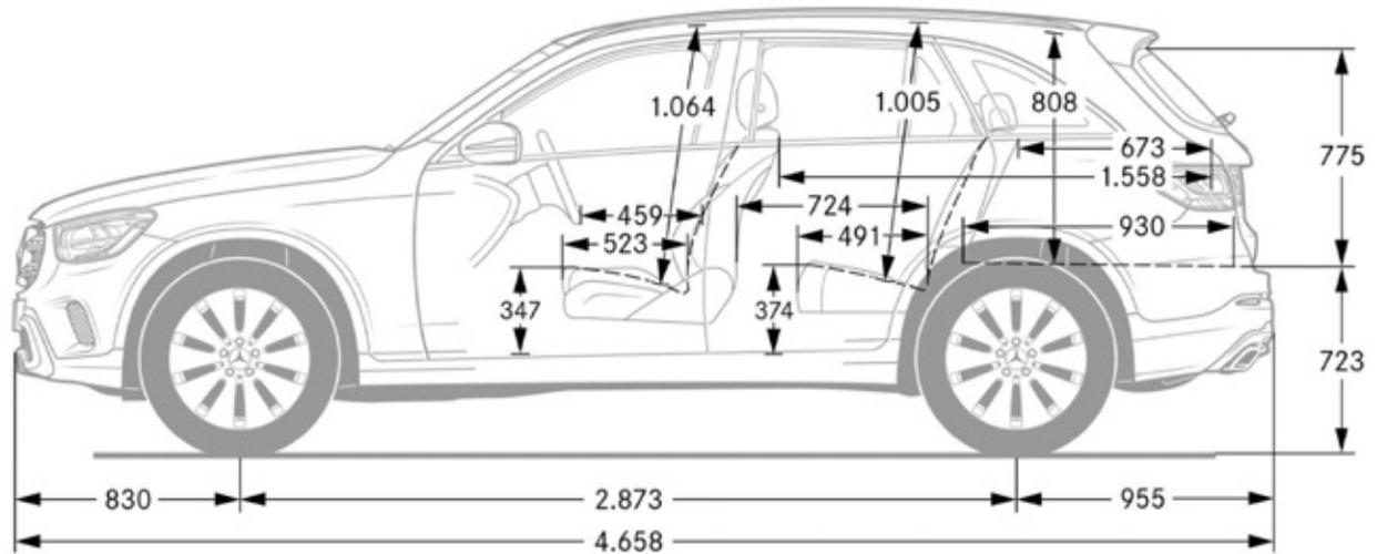
All dimensions in millimetres. The dimensions shown are mean values and apply to standard-specification, unladen vehicles.
