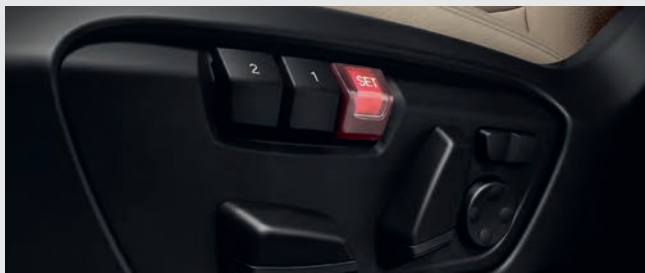
The Electric Seat Adjustment is easy to use and the memory function allows users to save their preferred settings for the seat and exterior mirrors.
