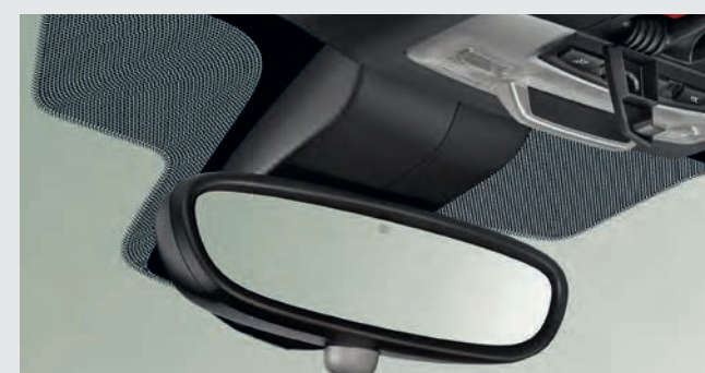
The interior mirror and driver-side exterior mirror feature the Automatic Anti-dazzle Function . Additionally, the driver-side exterior mirror features the automatic curb parking function when the vehicle is put in reverse. Both exterior mirrors are equipped with an electric folding function, as well as a mirror memory function. That makes parking easier and helps to avoid damage to the vehicle.
