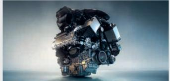
$\blacksquare$  The latest version of the high-performance BMW M TwinPower Turbo 8-cylinder petrol engine guarantees performance in keeping with the latest standards. The high-revving unit develops an output of 460 kW (625hp). The two turbochargers stand out thanks to their cross-cylinder bank exhaust manifold with optimum response characteristics. The V8 engine is also designed for extreme loads on the race track.
