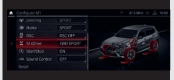
■ BMW M xDrive with Active M differential guarantees maximum traction and driving dynamics for everyday driving, as well as at the racetrack. The M specific technology combines the typical agility of a rear-wheel drive with the control of an all-wheel drive. You can choose between the two drive variants 4WD and 4WD Sport.
