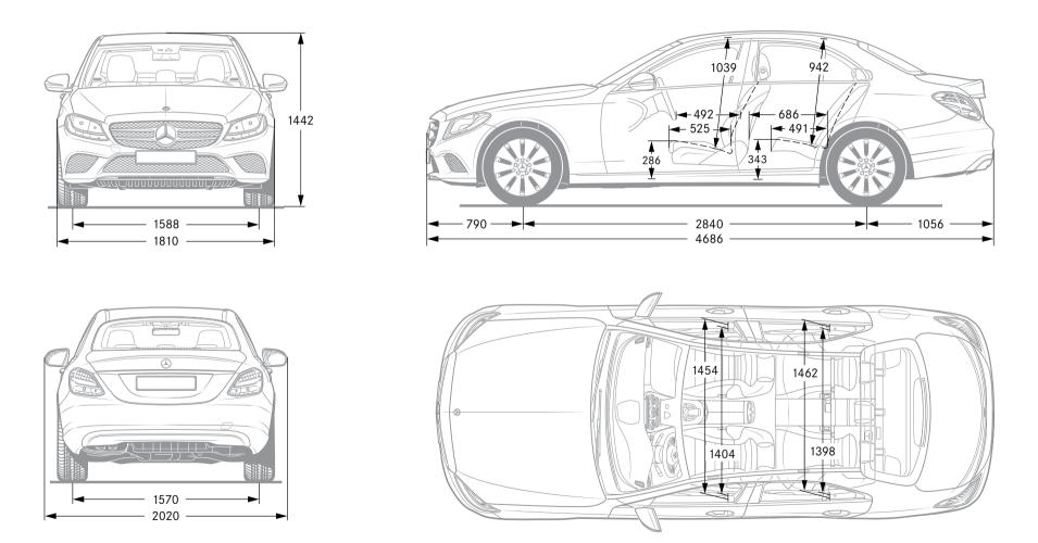
All figures in millimetres. The illustrated dimensions are mean values. They are valid for vehicles in basic specification and in unladen condition.
