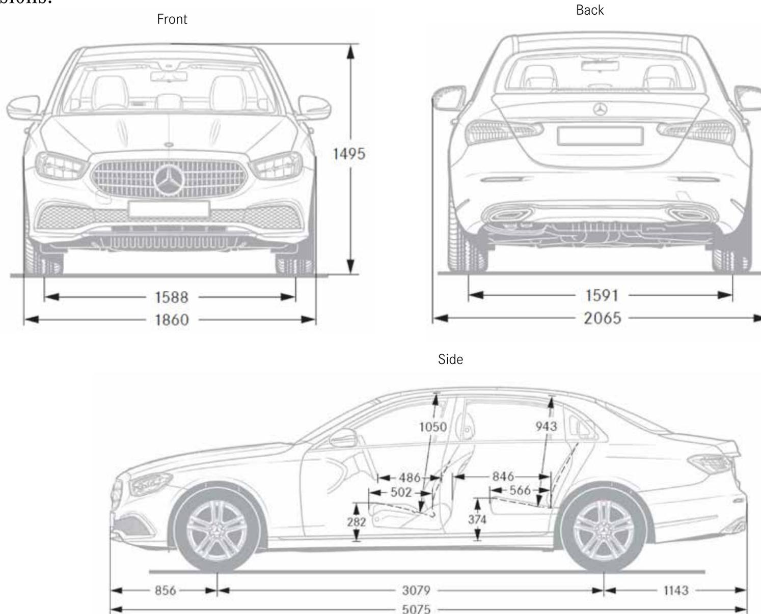
All measurements in millimetres. The dimensions shown are mean values and apply to standard-specification, unladen vehicles.
