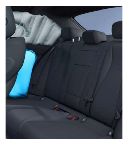
The side airbags in the rear protect the chest area on the outer rear seats in the event of a severe side impact. Together with the standard window airbags you therefore have optimum safety potential for preventing or lessening injuries. The air cushions slide between the side of the door and the occupant.
