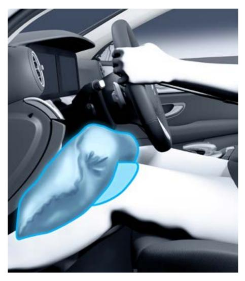
The knee airbag protects your legs from contact with the steering column or the dashboard in a severe frontal crash. This can prevent or lessen the severity of injuries. The air cushion inflates in milliseconds and stabilises the whole body. This ensures that the entire restraint system including the seat belt work together optimally.
