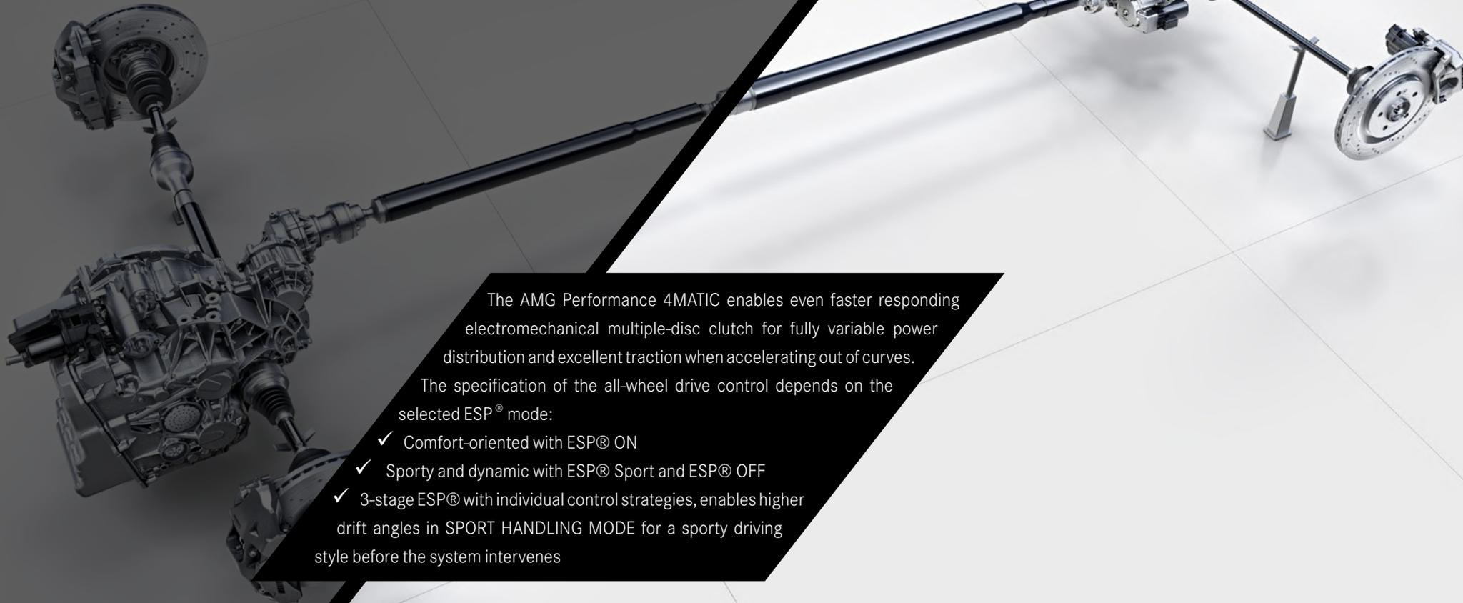
The AMG Performance 4MATIC enables even faster responding electromechanical multiple-disc clutch for fully variable power distribution and excellent traction when accelerating out of curves.
