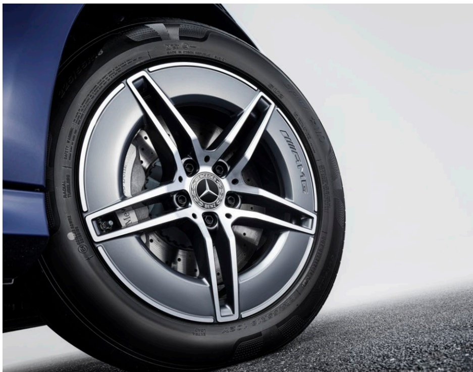
45.7 cm (18-inch) AMG 5-twin-spoke light-alloy wheels painted in tantalite gray with a high-sheen finish (Available with E 450 4MATIC)
