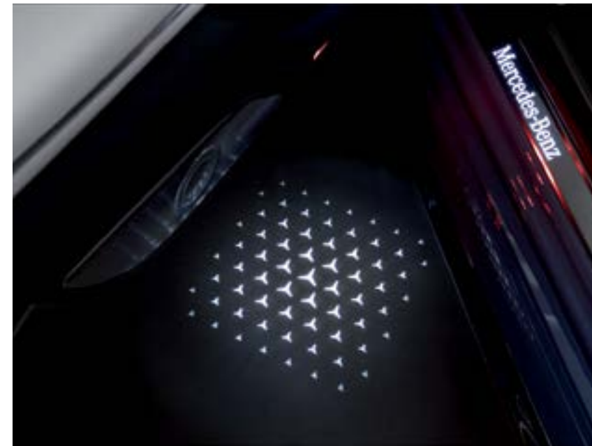
LCD projector with an animated Mercedes-Benz pattern for the rear doors
