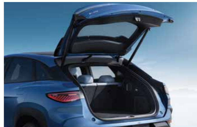
Kick Sensor Electrically Operated Trunk Gate
