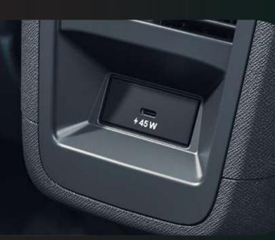
Front & rear fast charge C type 45W
