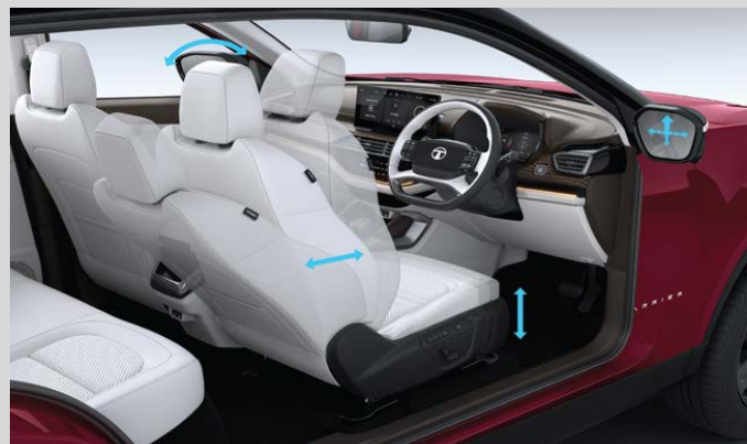
6 WAY POWERED DRIVER SEAT WITH MEMORY
