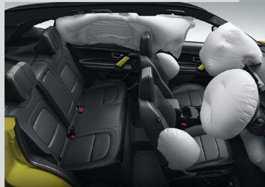
3-POINT ELR SEATBELT FOR ALL PASSENGERS | BUILT IN 7 AIRBAGS (6 STANDARD)
