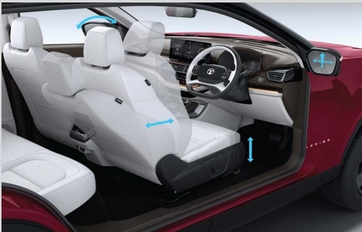
6 WAY POWERED DRIVER SEAT WITH MEMORY
