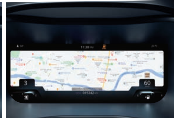
Navigation Display on Instrument Cluster
