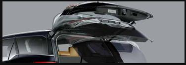
*Electronically Controlled Power Back Door with Memory* & Jam Protection
