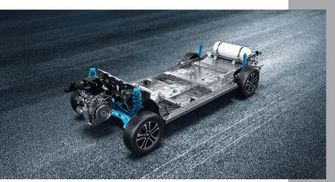
POWERFUL 1.5L (0.001462 m<sup>3</sup>) K SERIES ENGINE E-CNG technology for CNG grade | Fuel-efficiency of **26.11 km/kg**\* for CNG grade
