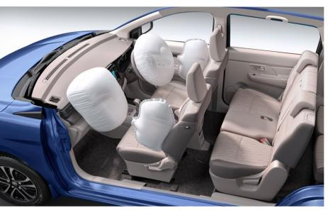
**DUAL FRONT AIRBAGS AND SEAT SIDE AIRBAGS FOR ENHANCED SAFETY**
