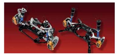
Handling duties are managed by a sophisticated 4-wheel independent suspension system mounted to high-precision 6-point front and rear subframes. A special Bilstein DampTronic driver adjustable shock absorber system utilizes multiple vehicle information systems to provide appropriate damping forces and a high level of control for a variety of driving situations.
