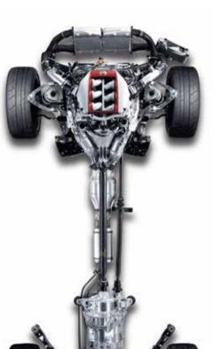
Dry Sump Lubrication System To ensure stable lubrication for the transmission even when cornering at high Gs, a dry sump lubrication system is employed. The system sprays transmission oil directly onto the gears, reducing friction and increasing reliability.
