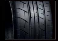
Even the design details of the GT-R's Dunlop SP Sport MAXX GT600 DSST CTT high-performance run-flat tyres are obsessive: a tiny block of rubber added to one of the treads combats tread squirm and gives a more confident, precise feel at the wheel.
