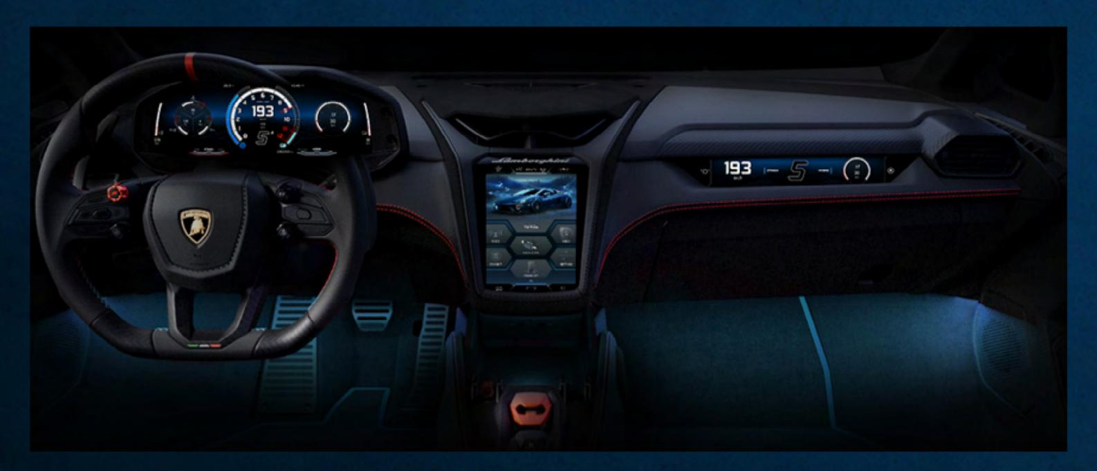
animations, and widgets. The new HMI is also highly customizable, offering three view options: "Dynamic View" for vehicle dynamics information, "Navi View" for a full-screen map, and "Essential View" for basic driving information. The Infotainment can be customized at will to create a fully immersive experience based on the user's preference.
