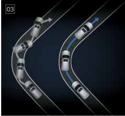
03 / Multi-terrain ABS with EBD The Multi-terrain ABS (Anti-lock Brake System) senses driving conditions on dirt or sand, and optimizes ABS control for excellent stopping performance on different road surfaces. EBD (Electronic Brake force Distribution) helps to optimize the application of braking force to each wheel.
