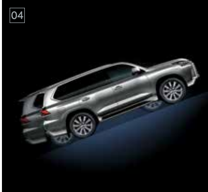
04 / Hill-start Assist Control When starting off on a slope, Hill-start Assist Control automatically maintains brake pressure to help prevent the vehicle from slipping backwards. It works both on-road and off-road to help reduce driver fatigue.
