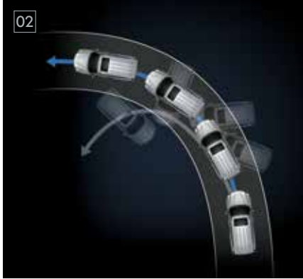
02 / VSC (Vehicle Stability Control) VSC helps prevent the loss of vehicle control, particularly when cornering quickly or at the onset of a skid. Selective application of the brakes and/or reducing power helps to enhance stability and reduce vehicle speed.
