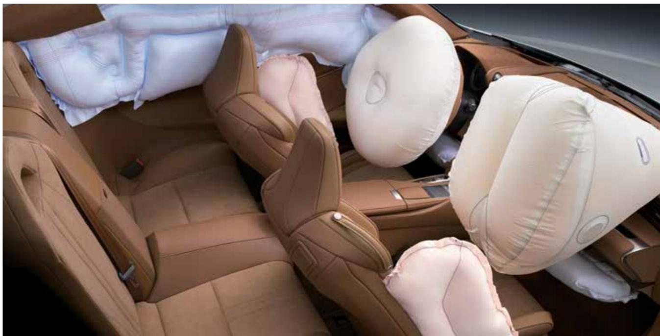
**SRS (Supplemental Restraint System) airbags**
