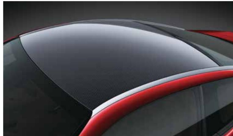
**CFRP (Carbon Fiber Reinforced Plastics) roof**
