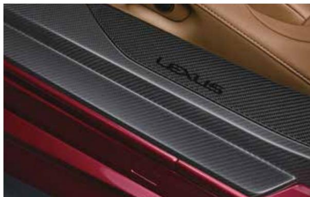
**CFRP (Carbon Fiber Reinforced Plastics) scuff plates**
