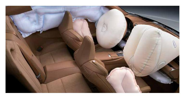
SRS (Supplemental Restraint System) airbags
