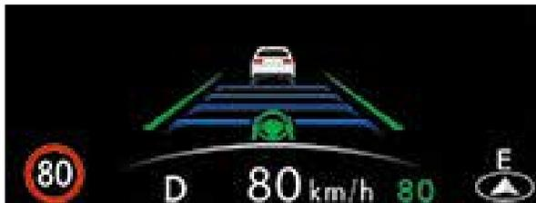
**Full:** Relaxed driving (when using driving assist systems, etc.) System operational status is displayed in a large, easy-to-understand manner.
