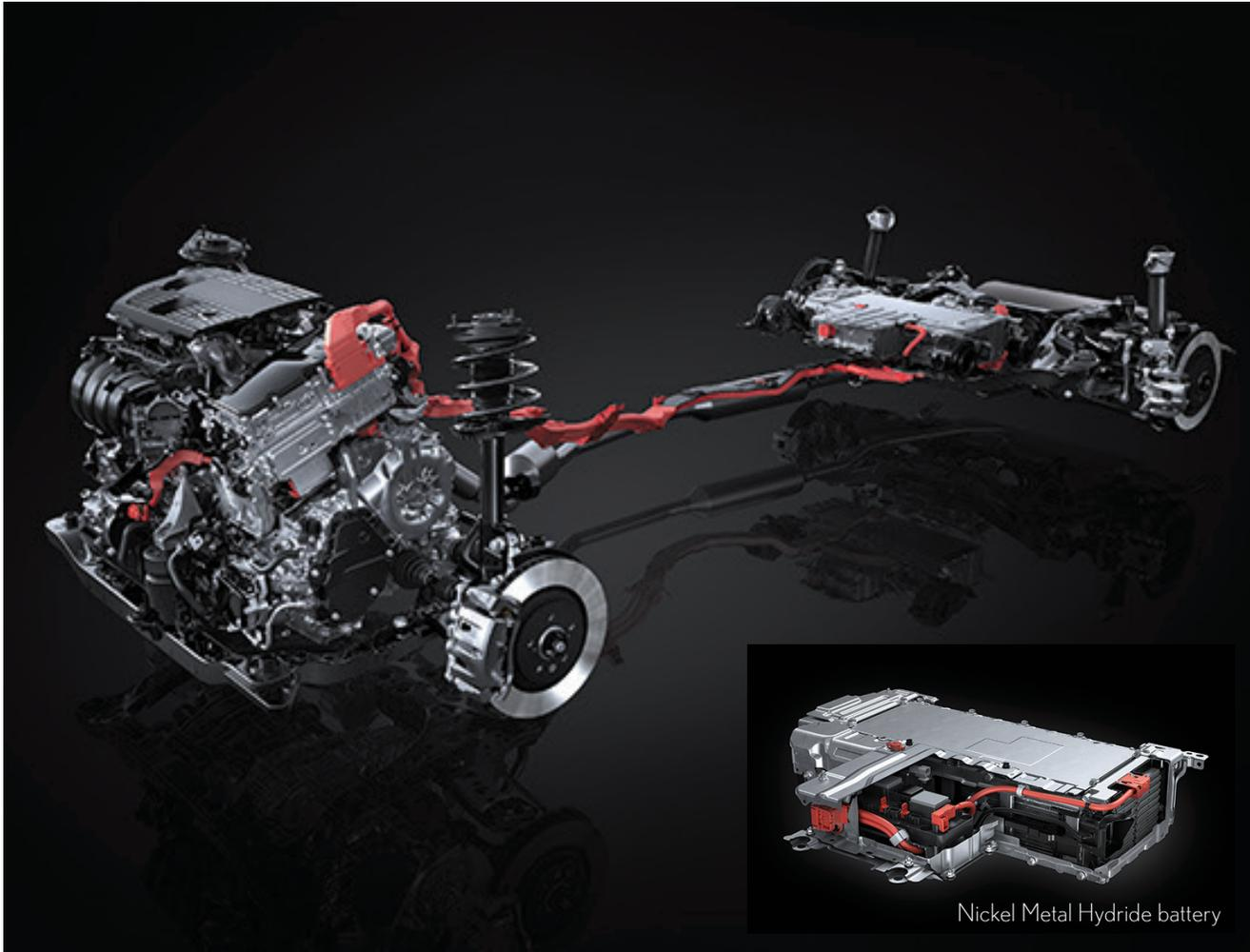
The hybrid system combines a highly efficient and responsive 2.5-liter inline 4-cylinder engine and high-output motor. A high-level balance between smooth, direct driving performance and excellent fuel economy has been enabled by effectively combining a highly responsive engine, bipolar nickel-metal hydride battery with enhanced battery performance, and hybrid system control with revised drive force characteristics.
