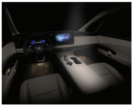
**FRONT SEATS** Indirect lighting is on the pull handle, e-Latch lever, and footwell.
