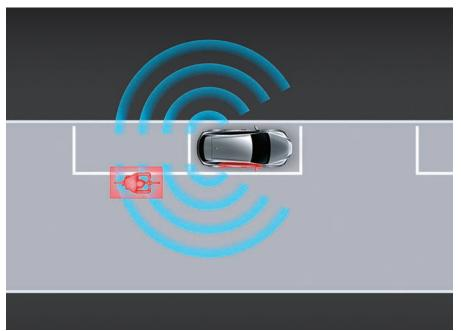
SEA uses the BSM (Blind Spot Monitor System) to detect vehicles or bicycles approaching from the rear, when exiting the vehicle. If SEA determines a collision with an opened door or exiting occupants is a possibility, an indicator in the door mirror lights up to alert occupants. In addition, if an occupant tries to open a door, the e-latch system cancels door unlatch operations. Occupants are alerted by flashing indicators in the door mirror, the multi-information display, and a buzzer.
