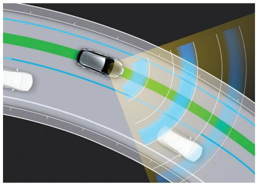
Lane recognition performance has been enhanced to realize smoother and less disruptive steering support. In situations such as overtaking a vehicle in the adjacent lane, or when there is a close distance between the vehicle and an off-road structure, the tracing position is offset from the center of the road to the avoidance side, just like the driver's driving, to achieve cooperative control with the driver.
