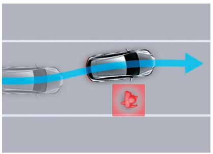
LDA works in tandem with the driver. For example, it deactivates the lane departure warning and restraint functions when it can judge that the driver has made a deliberate manoeuver to avoid a person or parked vehicle. In addition, the system now recognizes utility poles, curbs, guardrails, walls, and continuous poles, enabling additional support at lower speeds.
