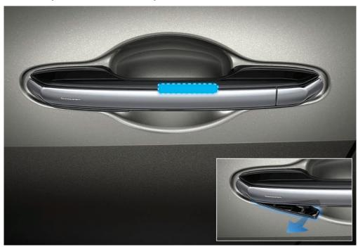
An e-latch system replaces the conventional door latch/unlatch mechanism with an electronic control that opens and closes doors smoothly with no wasted movements, like a sliding shoji paper door.
