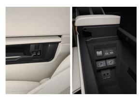
**PERSONAL CHARGING STATIONS** A Qi-wireless charging station and two USB Type-C ports are located next to the seats' outer armrest within the covered quarter box. A headphone socket is also included.
