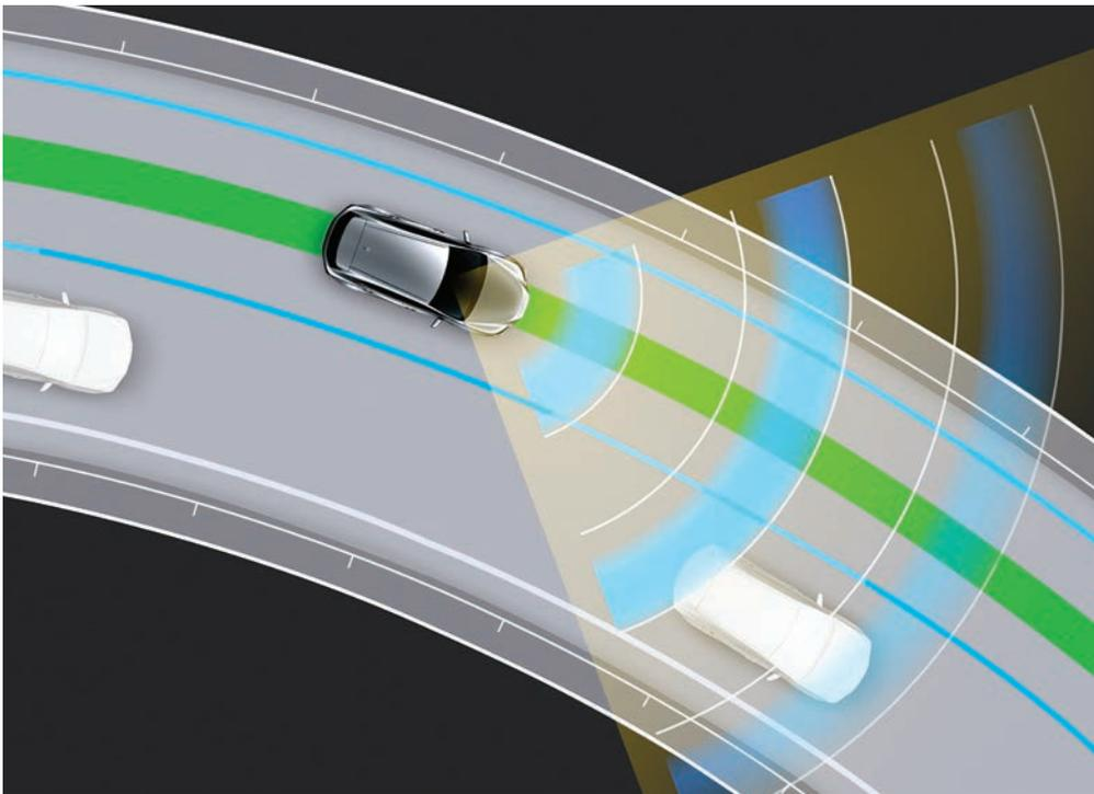
Lane recognition performance has been enhanced to realize smoother and less disruptive steering support. In situations such as overtaking a vehicle in the adjacent lane, or when there is a close distance between the vehicle and an off-road structure, the tracing position is offset from the center of the road to the avoidance side, just like the driver's driving, to achieve cooperative control with the driver.
