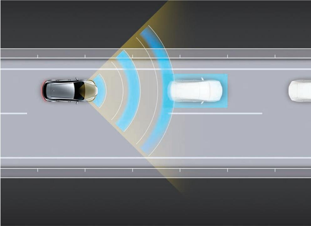
In addition to providing preliminary acceleration in response to the operation of the turn signal when overtaking another vehicle, if a preceding vehicle in the target lane is traveling at a speed slower than the set vehicle speed, the system provides preliminary deceleration, again in response to the operation of the turn signal. This prevents a sudden approach to the preceding vehicle and enhances the sense of security.
