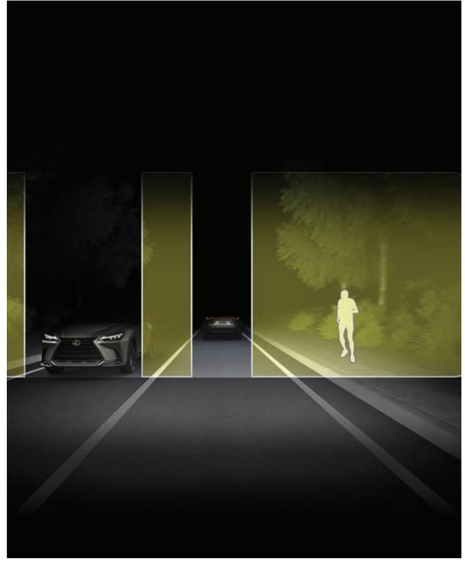
Headlamp light distribution is automatically adjusted once light from an approaching or preceding vehicle is detected by a monocular camera. Twelve independent LED chips within the headlamps can be enabled/disabled for precise control of illuminated or non-illuminated areas.
