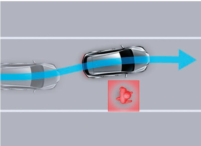
LDA works in tandem with the driver. For example, it deactivates the lane departure warning and restraint functions when it can judge that the driver has made a deliberate manoeuvre to avoid a person or parked vehicle. In addition, the system now recognizes utility poles, curbs, guardrails, walls, and continuous poles, enabling additional support at lower speeds.
