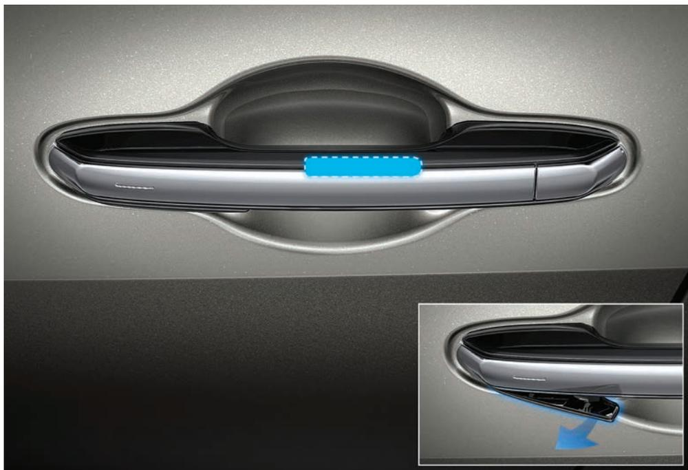
An e-latch system replaces the conventional door latch/unlatch mechanism with an electronic control that opens and closes doors smoothly with no wasted movements, like a sliding shoji paper door.
