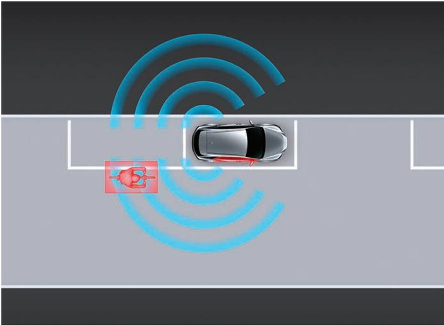
SEA uses the BSM (Blind Spot Monitor System) to detect vehicles or bicycles approaching from the rear, when exiting the vehicle. If SEA determines a collision with an opened door or exiting occupants is a possibility, an indicator in the door mirror lights up to alert occupants. In addition, if an occupant tries to open a door, the e-latch system cancels door unlatch operations. Occupants are alerted by flashing indicators in the door mirror, the multi-information display, and a buzzer.
