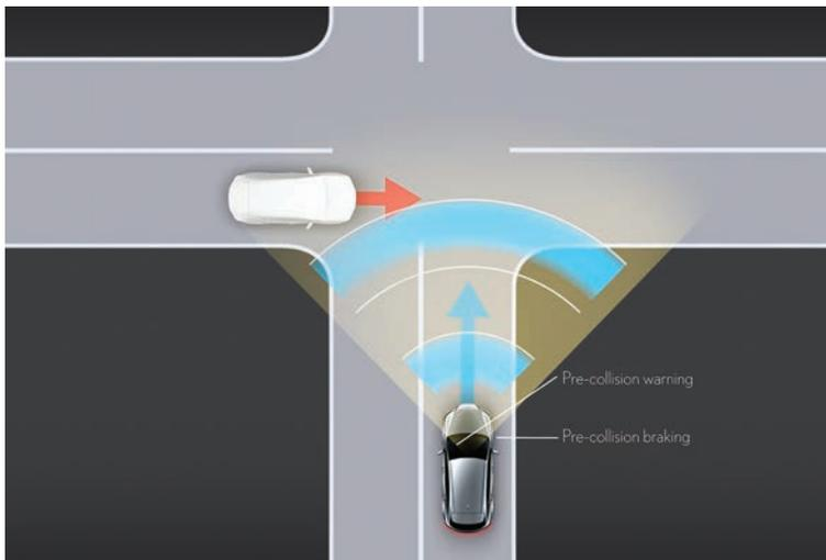
When the millimetre-wave radar and monocular camera sensors detect a vehicle ahead and determine that a collision is likely, it alerts the driver with a buzzer and on the display. If the system determines that a collision is likely, it alerts the driver and activates the brake support to help mitigate damage.
