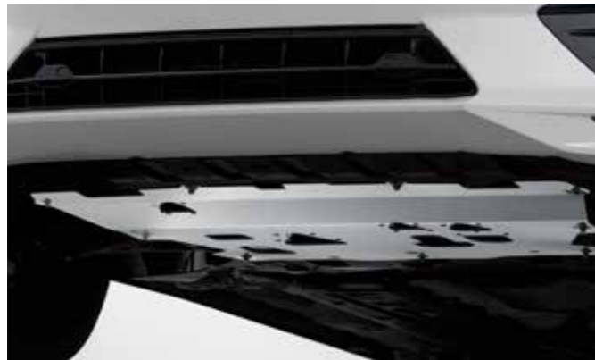
Protective Plate Beneath Engine.
