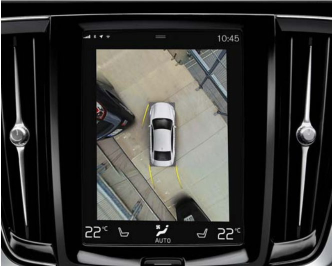
360° camera The 360° camera uses images from discreetly mounted cameras to create a bird's eye view of your car and its closest surroundings. In the centre display, you can see obstacles all around you, which makes it easier to park and manoeuvre in tight spaces.
