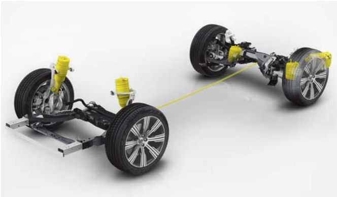
Air suspension on all four wheels gives the XC90 outstanding ride comfort – the air springs absorb up imperfections in the road – and make the car stable by keeping the ride height constant, regardless of the load. With the active chassis you can alter the way the car rides and handles to suit your mood or the road.
