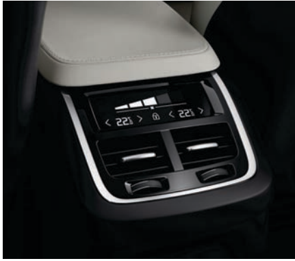
The four-zone climate system can be controlled from the centre display touch screen, or a graceful touch control panel at the end of the tunnel console.
