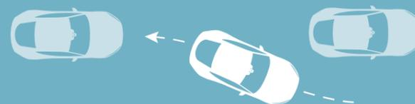
**Park Assist** (Optional) can help make parking easier by steering your vehicle into and out of a suitable space. After selecting either Drive or Reverse, you only have to control the vehicle's speed and braking. Graphics and notifications will guide you through the manoeuvres.
