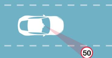
**Lane Keep Assist** detects when the vehicle is unintentionally drifting out of the lane, and applies corrective torque to the steering wheel, encouraging you to guide your vehicle back.
