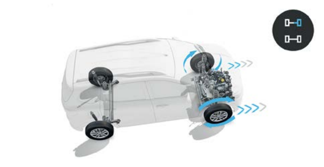
traction control system Limits wheel slip during starting, acceleration and braking.
