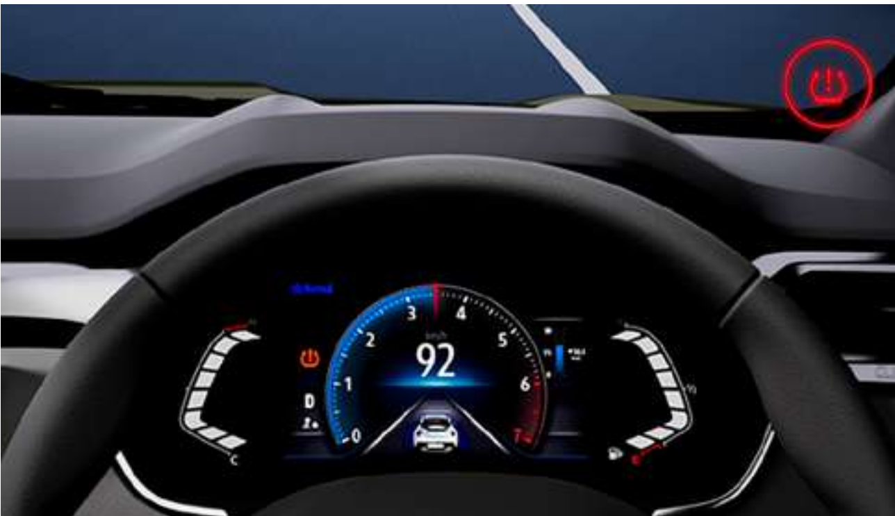
tyre pressure monitoring system Displays the tire pressure status in real-time.
