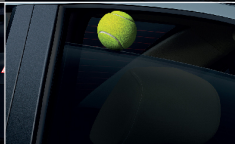
DRIVER SIDE WINDOW ONE TOUCH UP/ DOWN WITH PINCH GUARD
