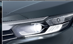
NEW AUTOMATIC HEADLIGHT CONTROL WITH LIGHT SENSOR
