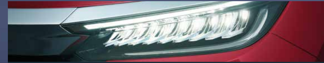
Full LED Headlamps (with 9 array Inline Shell, Integrated LED DRL, L-Shaped Turn Signal)
