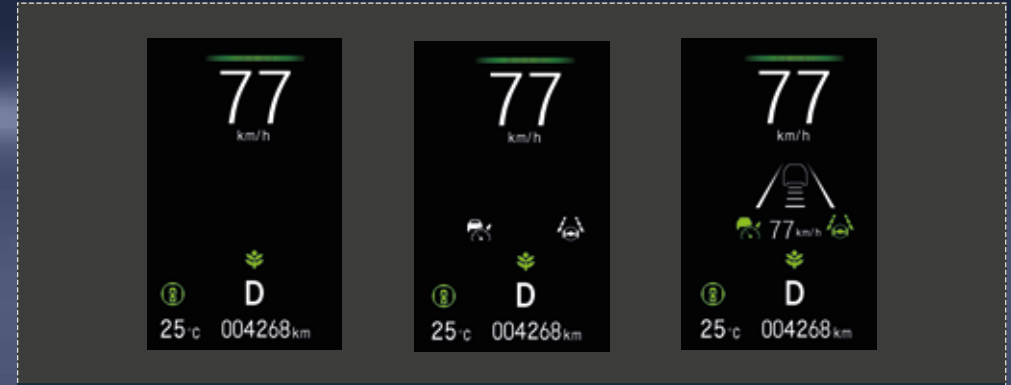
Adaptive Cruise Control Visual Display, CMBS & RDM Status, Digital Speed Display
