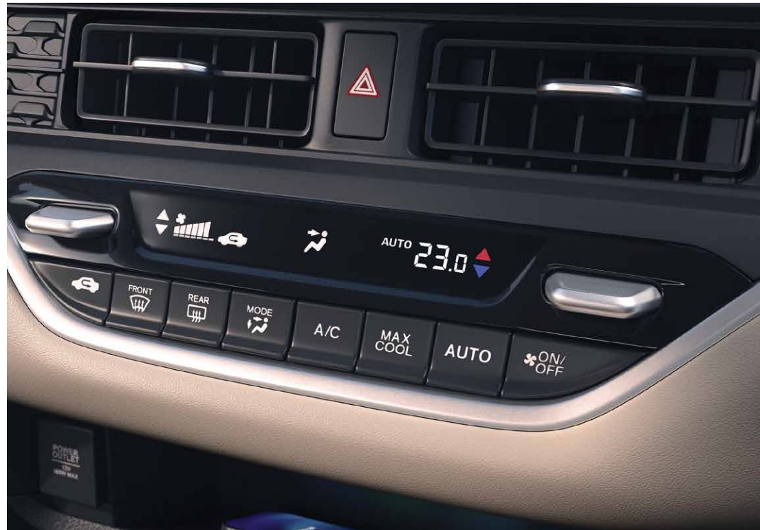
FULLY AUTOMATIC CLIMATE CONTROL WITH MAX COOL
