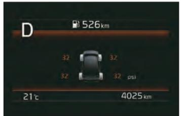
Continuously monitors air pressure in each tyre and alerts you in case of a drop below recommended levels
