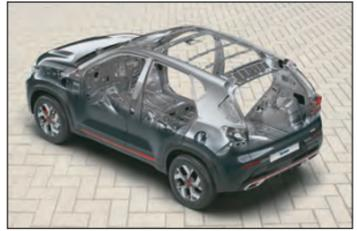
Offers enhanced safety as more than 2/3<sup>rd</sup> of structure is made from high strength steel
