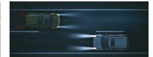
automatically adjusts the high beam/ low beam based on the oncoming vehicle's headlamp intensity
