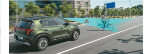
alerts the driver of imminent collision with any cyclists ahead and applies brake
