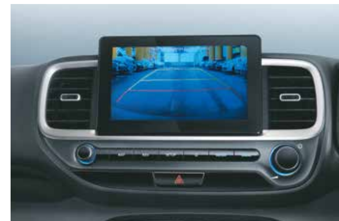
Rear parking assist system
