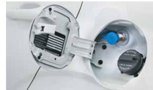
Convenient CNG filling valve location near petrol fill area
