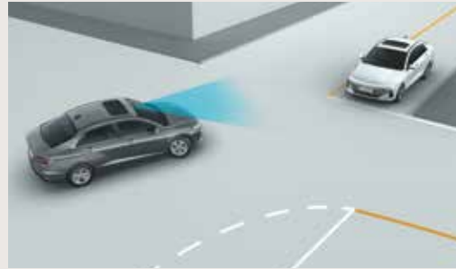
Forward Collision - Avoidance Assist - Junction Turning (FCA-JT)
