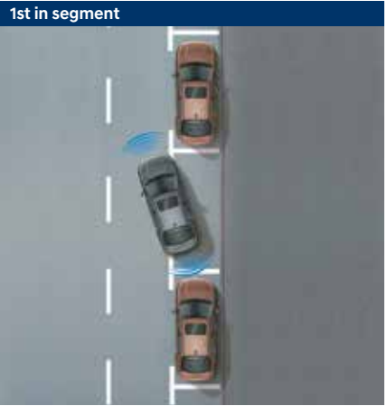
Parking assist (front & rear parking sensors and rear camera with guidelines)
