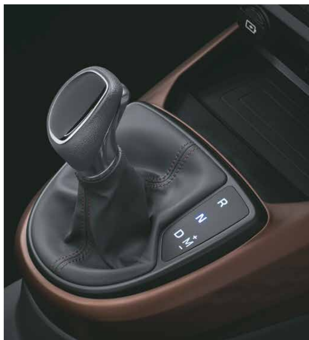
Automated manual transmission (AMT)
