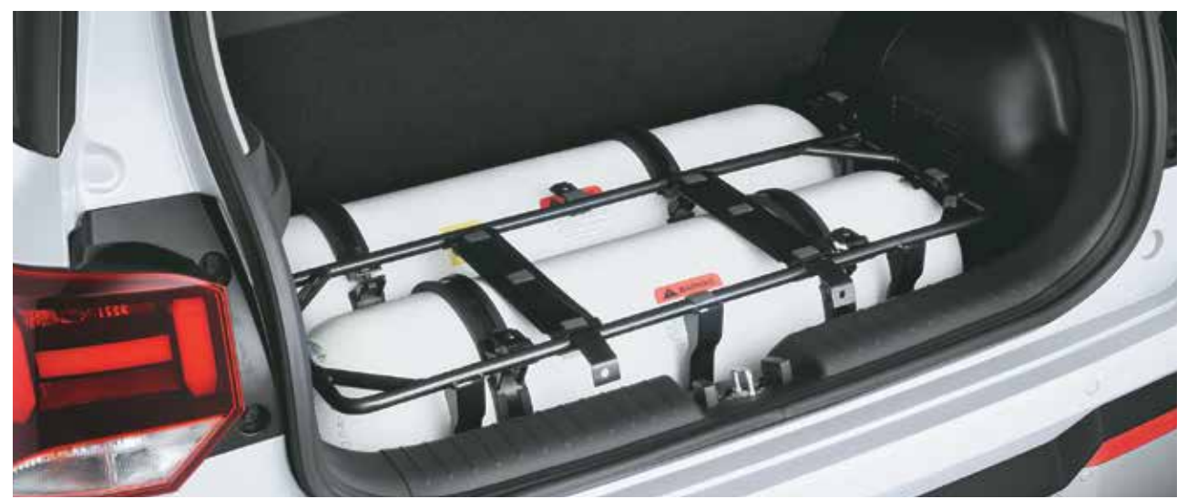
Company fitted dual cylinder CNG
