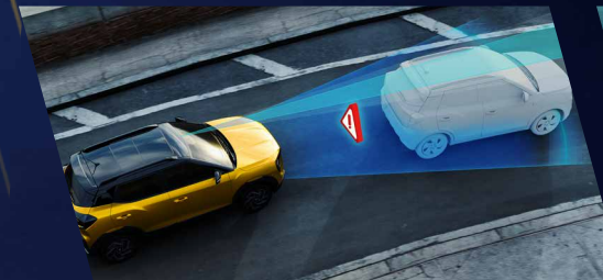
Forward Collision Warning
