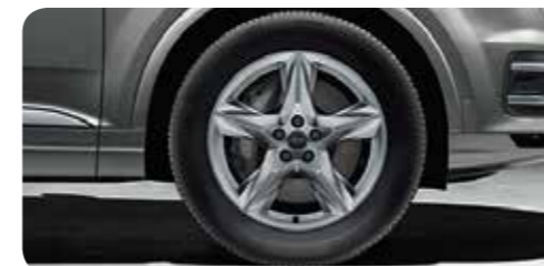
Cast aluminium wheels in 5-spoke star design* size 8.5 J x 48.26cms with 255/55 R 19 tyres
