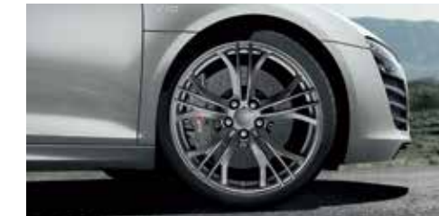
Forged aluminium wheels in 5-twin-spoke Y design* in titanium look size 8.5 J x 19 at front and 11 J x 19 at rear, with 235/35 R 19 tyres at front and 305/30 R 19 tyres at rear
