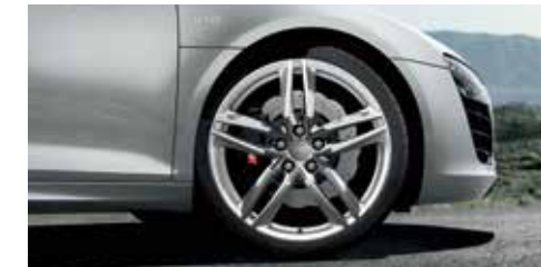
Forged aluminium wheels in 5-twin-spoke design*, high-gloss polished size 8.5 J x 19 at front and 11 J x 19 at rear, with 235/35 R 19 tyres at front and 305/30 R 19 tyres at rear
