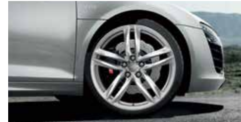
Cast aluminium wheels in 6-arm design, (V8) Size 8.5 J x 18 at front, size 10.5 J x 18 at rear, with 235/40 R18 tyres at front and 285/35 R18 tyres at rear
