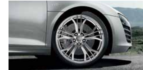
Forged aluminium wheels in 5-twin-spoke Y design* size 8.5 J x 19 at front and 11 J x 19 at rear, with 235/35 R 19 tyres at front and 295/30 R 19 tyres at rear
