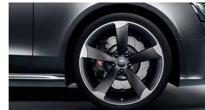
Cast aluminium wheels* in 5-arm rotor design in titanium look, high-gloss turned finish size 9 J x 20 with 275/30 R 20 tyres
