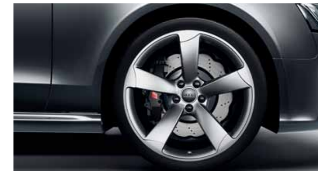
Cast aluminium wheels* in 5-arm rotor design size 9 J x 20 with 275/30 R 20 tyres
