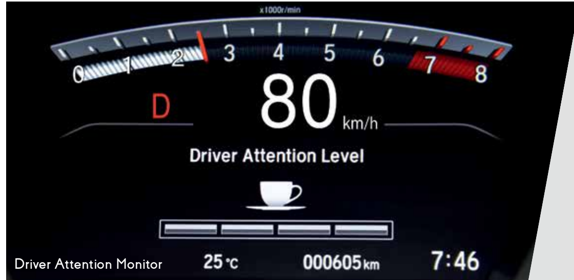
Driver Attention Monitor Alerts you with sound and vibration when it detects low level of alertness.
