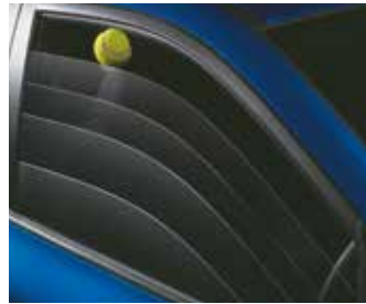
Auto Up/Down Power Window with Pinch Guard
