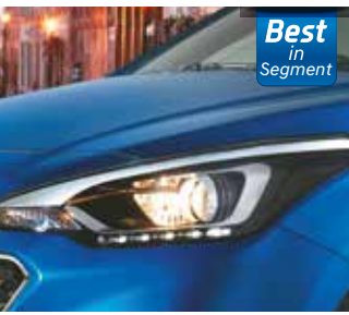
Projector Headlamps with LED DRL, Positioning and Cornering Lamps
